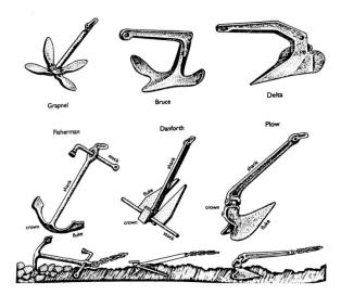
weight of the chain the holds the vessel. This is why it is important to have plenty of scope when anchoring. It is recommended to have 5-7 times the length of scope to depth of the water. There for if you are anchoring 40 feet of water, you should have a minimum of 200 feet of scope.
