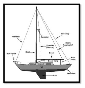
backstays, which are used when no permanent backstay can be fitted or when extra bracing is needed.
